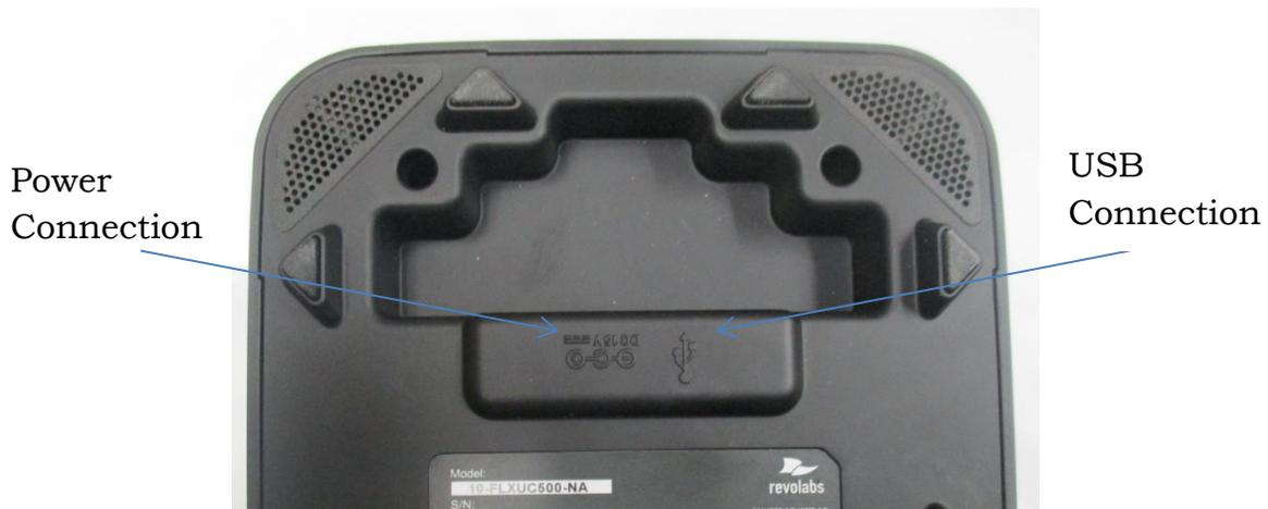
Figure 2: FLX UC 500, Connector View
